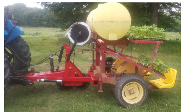
The no-till planter in action, attached to a tractor and filled with plants and water. The process of this planter limits disturbance to the soil environment.
